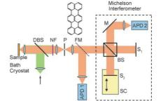
Single-molecule optical Fourier transform spectroscopy in combination with confocal microscopy is used for the first time for Raman and fluorescence studies of spatially isolated single-walled carbon nanotubes and single terrylene molecules. The picture shows a schematic diagram of the optical setup that was used to measure two beam interferograms from molecular emission.
